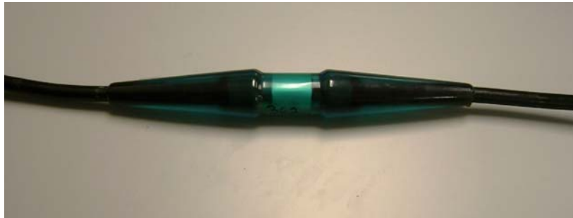
Figure 2. Array cable with hydrophone element and preamplifier pod.
