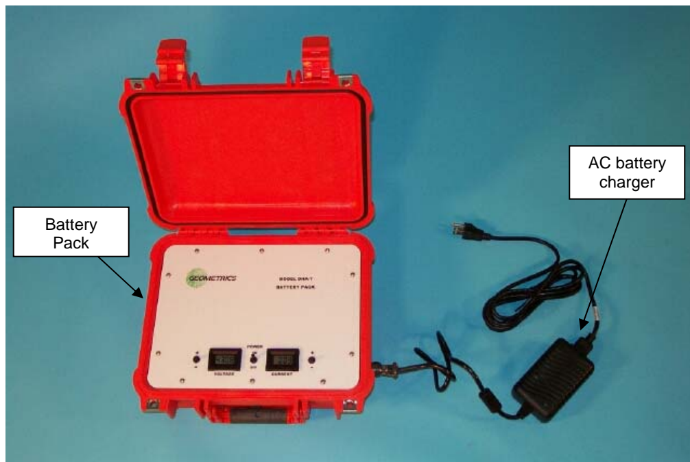
Figure 6. DHA-7/MicroEel Battery Pack with AC battery charger.
