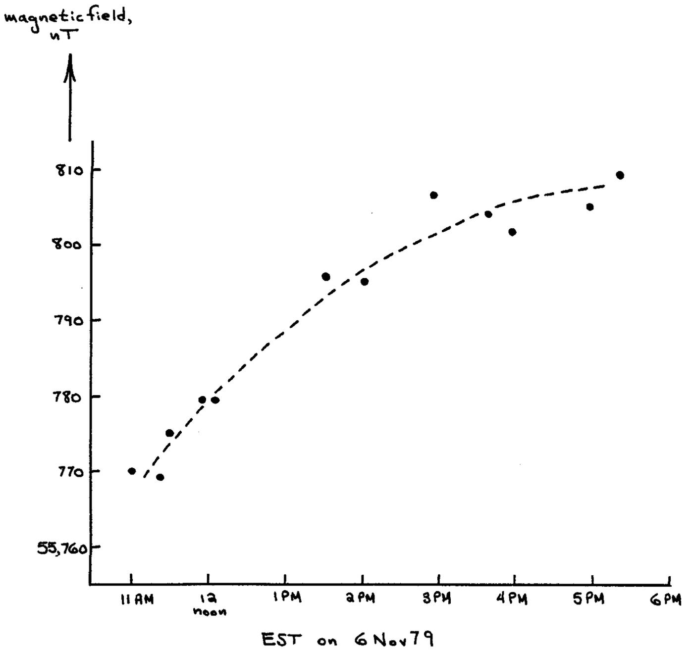
Diurnal change measured with cesium sensor resting on stake ~20cm above soil at point N30W10 of coordinate system "B".
