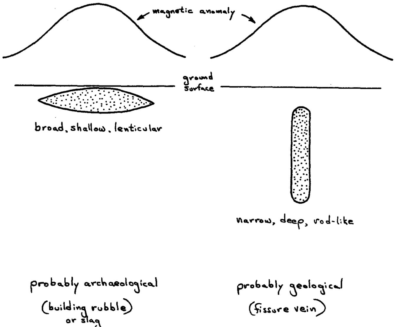
Figure 3: Different structures can cause similar anomalies
