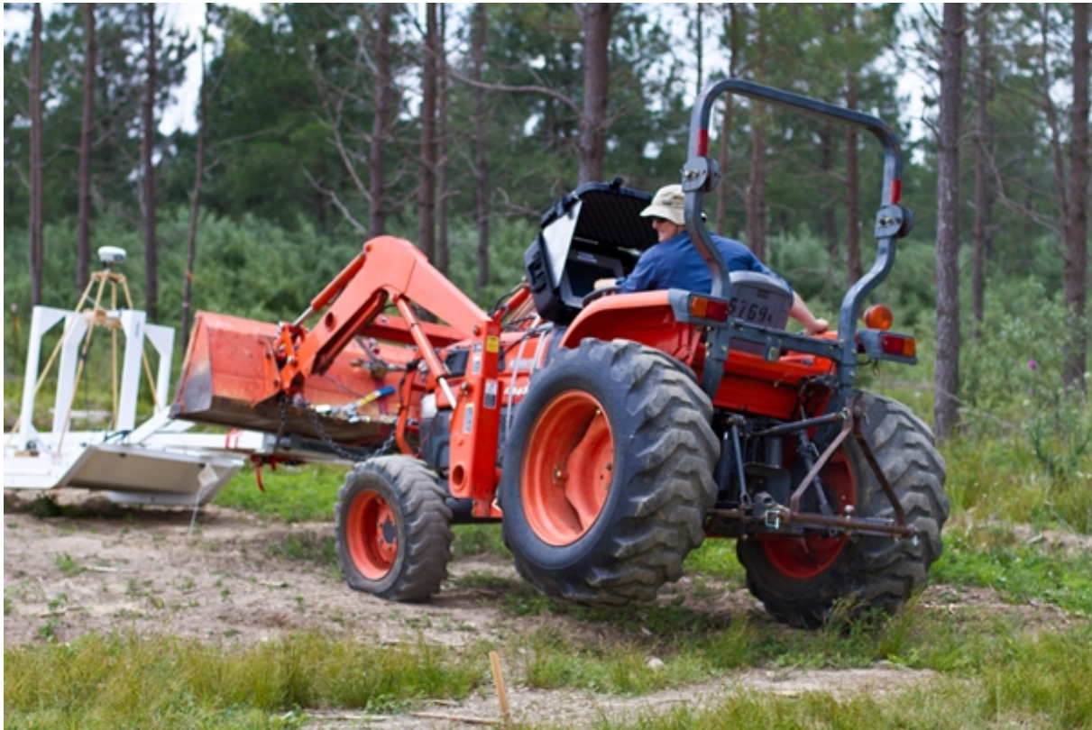
Figure 30. Tractor Instability while Raising MM
