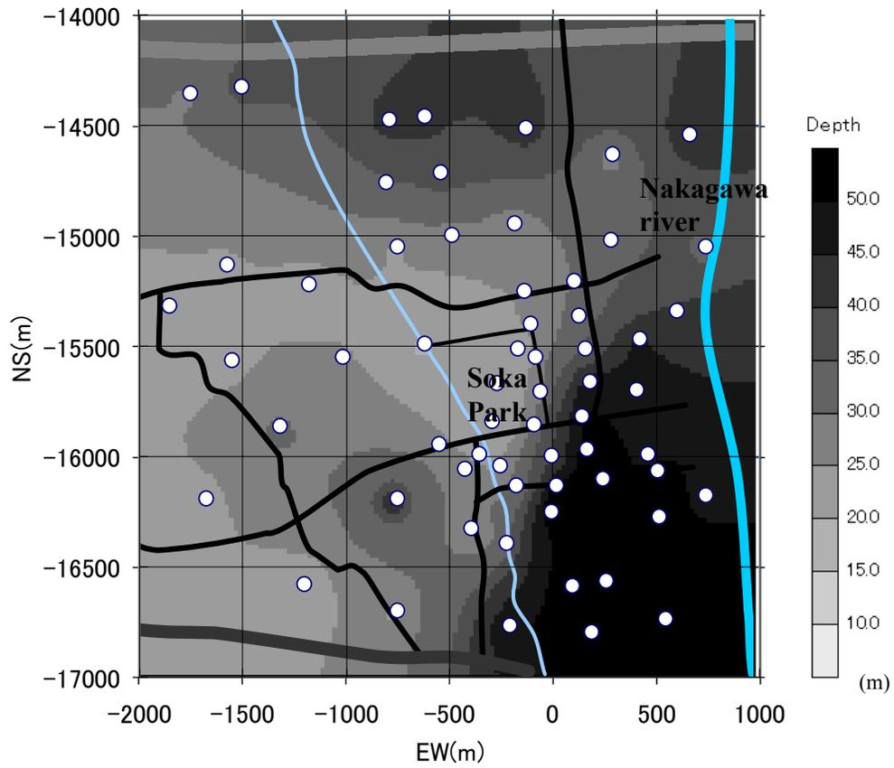
**Figure 7.:** Depth of alluvium bottom obtained through the survey.
