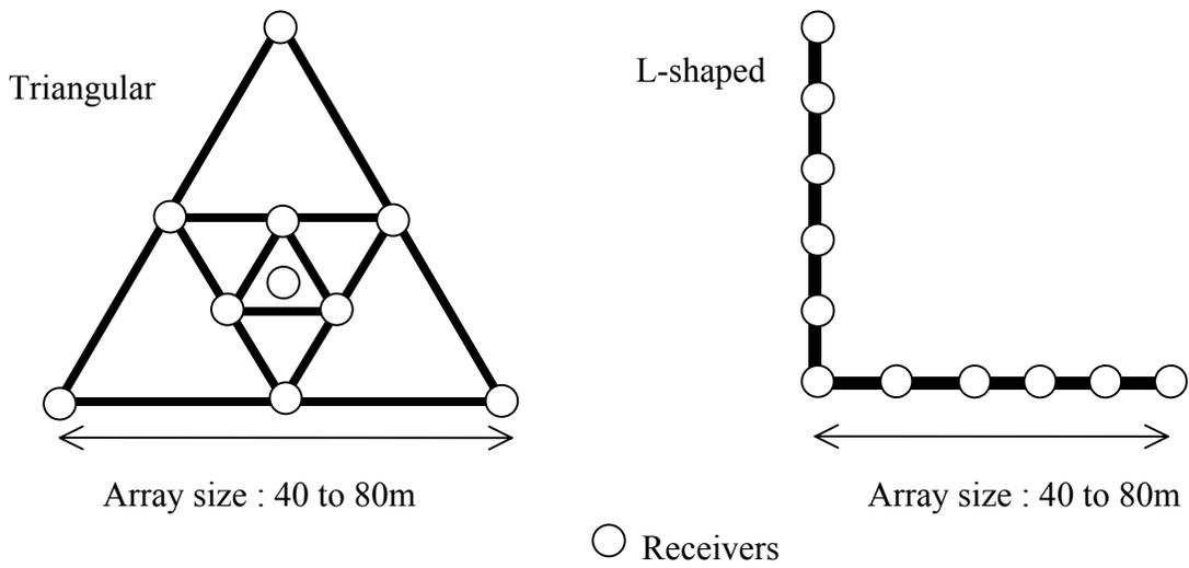
**Figure 3.:** Receiver arrays used in the passive method.
