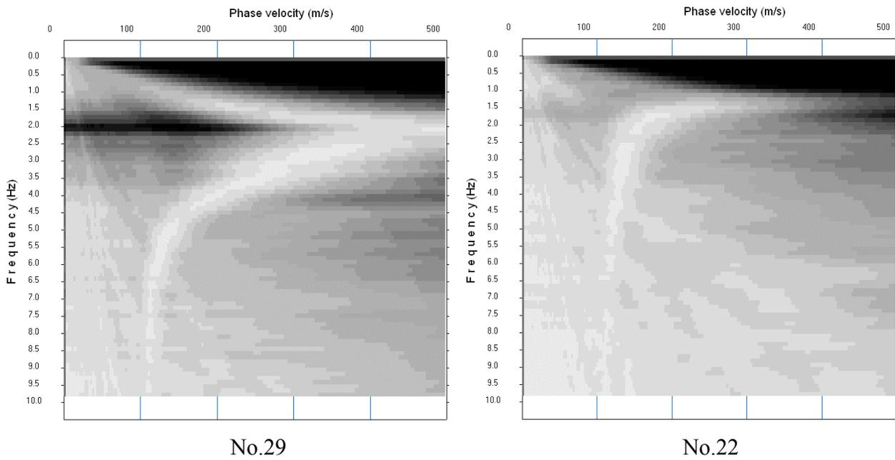
**Figure 4.:** Example of image of phase velocity versus frequency.
