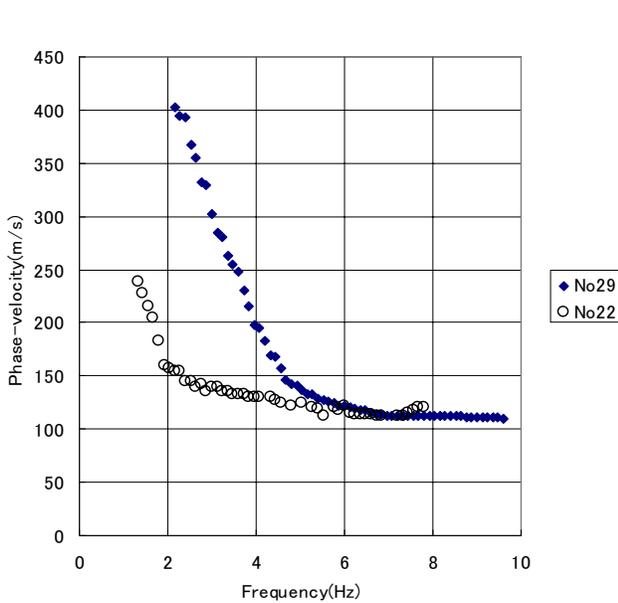
**Figure 5.:** Phase velocity curves on terrace (No.29) and in channel (no.22).
