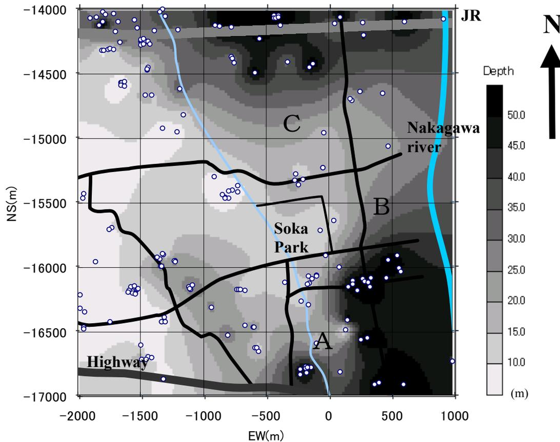
**Figure 1.:** Location of existing boreholes (white circles) estimated depth of alluvium.
