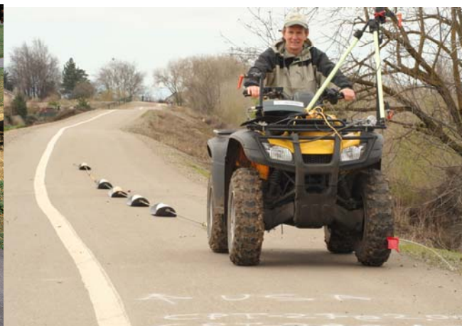
Figure 4b: Five-receiver vehicle-towed array
