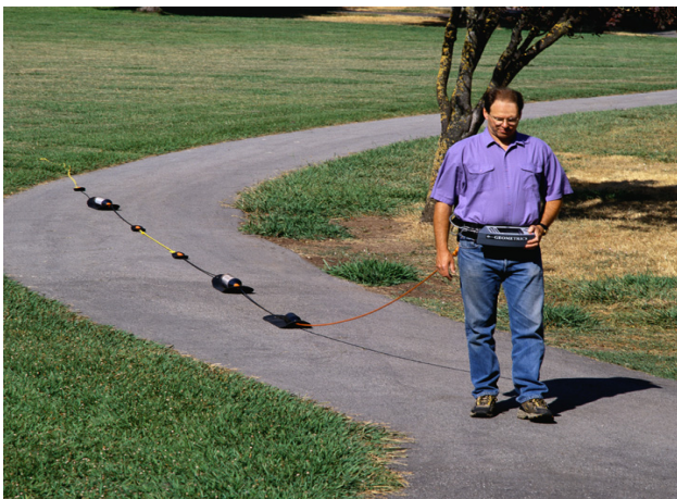
Figure 4a: Single-receiver manually-towed array
